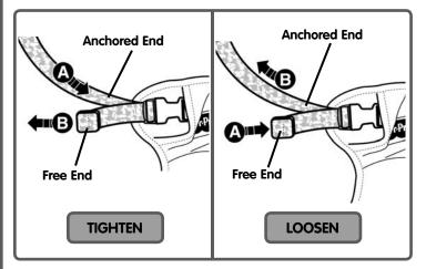
**To tighten the belts:** Feed the anchored end of the restraint up through the buckle to form a loop **Q**. Pull the free end of the restraint **G**.
